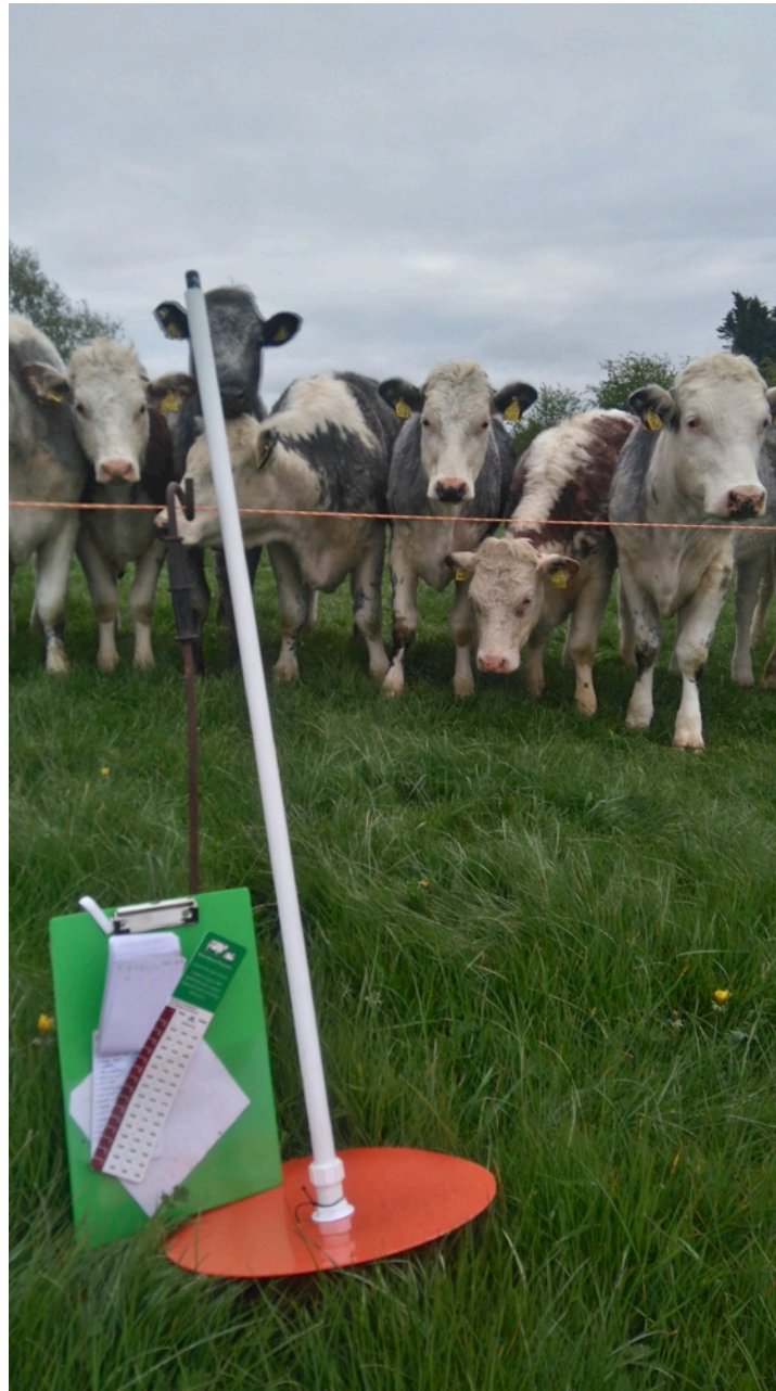
DIY Plate meter Its basic, its fully manual, but it works and is cheap.
